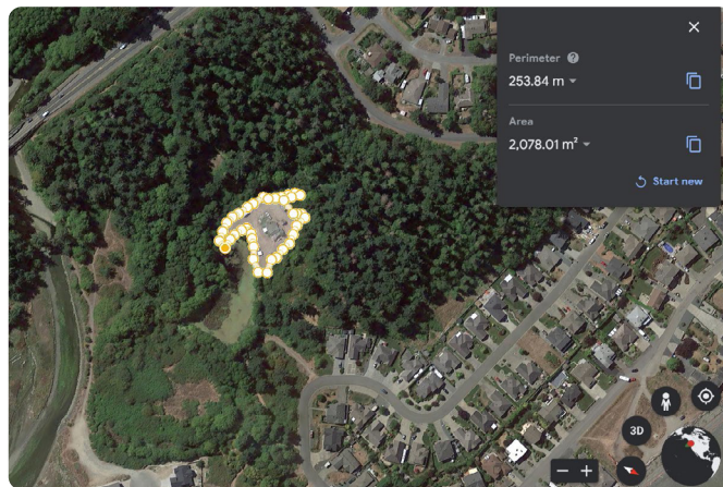
Fig. 2. A clearing in the French Creek Estuary Nature Preserve was outlined on Google Earth to calculate its area using the platform's measurement tool. This area can be repeatedly measured in subsequent years to track the rate of vegetation regrowth in the clearing. Image from 2019
